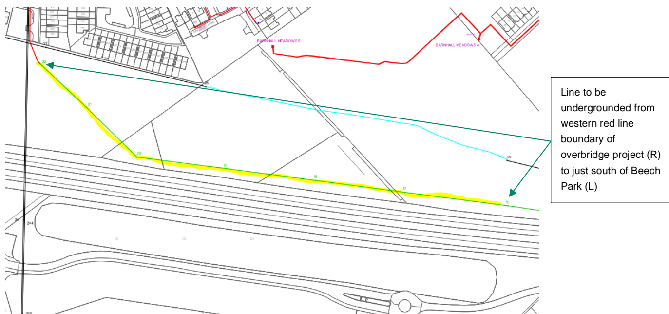
Figure 8. Extent of 10kV line to be undergrounded as part of the Wonderful Barn project
